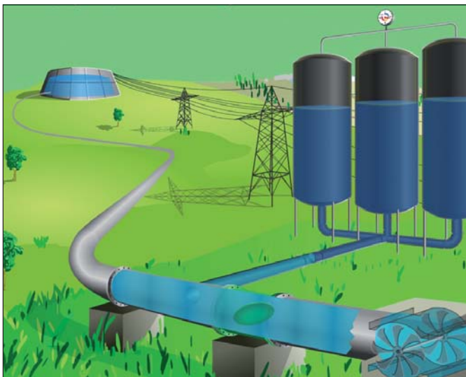
Surge vessel under operation of the pump
