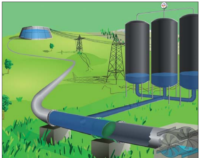
Surge vessel after a pump failure; the water equalises the vacuum
