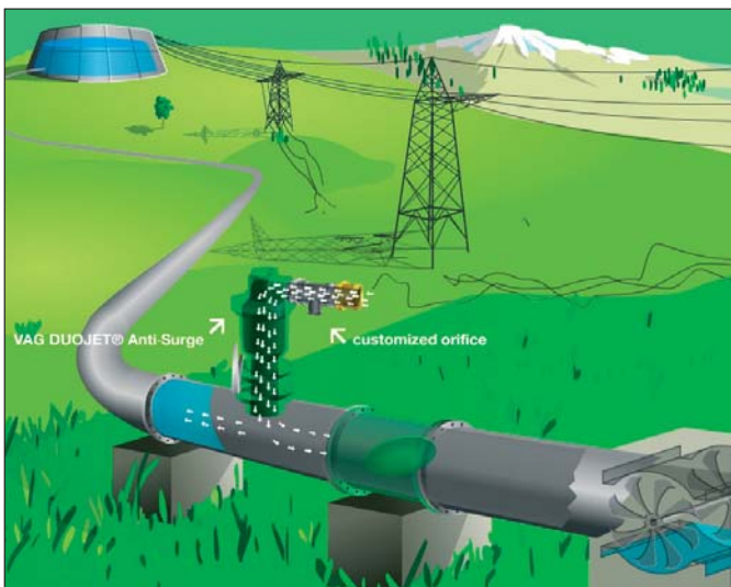
The VAG solution: After a pump trip / shut off, air equalises the vacuum which has developed
